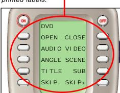
Up to 40 screen labeled buttons are available for each device. To view the additional buttons, press the PAGE button to display additional pages. The the remote control can display up to four pages of screen labeled buttons for each activity or device! As you scroll through the pages, notice that the bottom title bar displays which page you are viewing (PAGE 1, PAGE 2, etc.).
